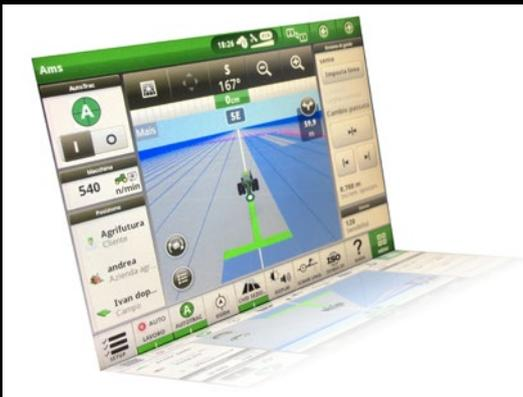
Once the prescription maps have been loaded into the ISOBUS monitor via USB, the tractor terminal obtains all the information regarding the rate of seed to deliver in each area.
