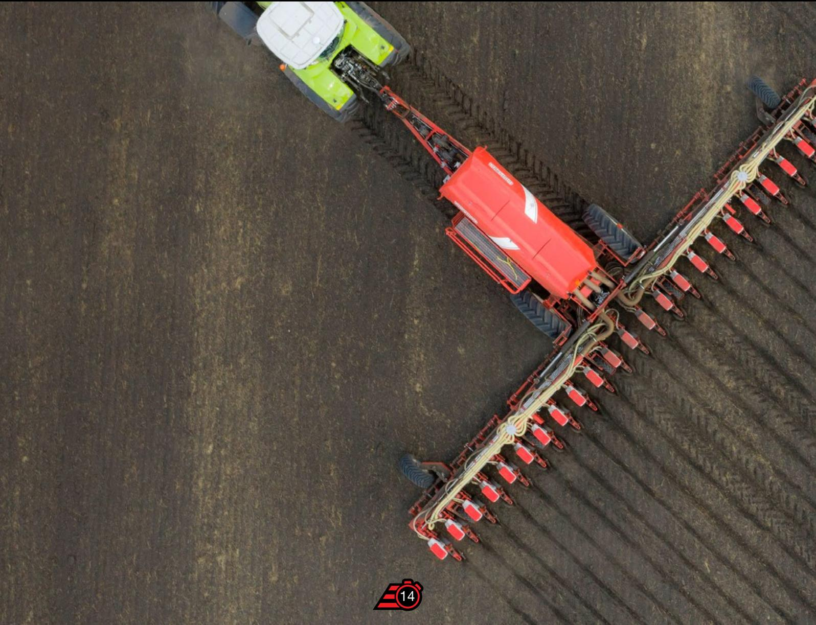
After exiting the distributor, the seed enters the new pneumatic system and it is transported into the ground through the air flow avoiding the negative bouncing effect. The seed counter is integrated on the seed tube and controls the seed delivery, while the soft rubber and self-cleaning press wheel holds the seed in the furrow, guaranteeing the best seeding accuracy and excellent depth consistency.
